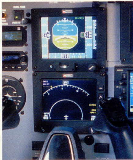
The Meggitt PFD shows about everything you need to fly the Meridian. The navigational display below improves situational awareness.
