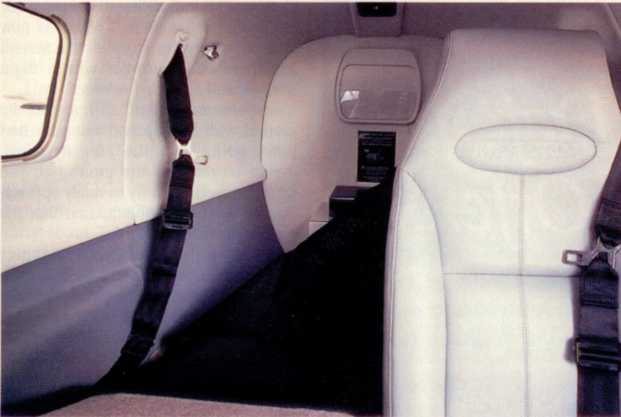
The aft seat backs are certified to bear weight when folded forward and when using a cargo net. Interior cabinets and materials are equivalent to what you might find in a business jet.
